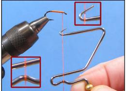
Come in with the tool from behind. Catch the thread with the top hook and the dent in the lower bend.
